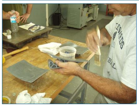
9. Apply 2 coats of the adhesive to the snaps and hook, using a 2" (50.8mm) soft bristle paint brush, with the bristles trimmed to 3/4" - 1" (19 - 25.4mm) long.
