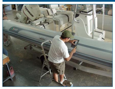
14. Insure that the bonding surfaces of the snaps and hook are fully seated to the bonding surfaces of the boat, that there are no voids or air pockets between the snaps and hook and the bonding surfaces of the boat.
