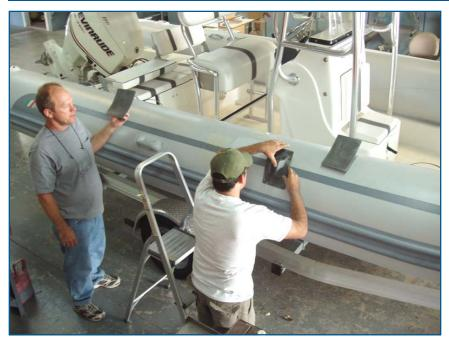
11. Starting at the bottom edge of the bonding surface, press the snaps and hook onto the boat surface with firm pressure, applying the pressure evenly from the bottom to the top of the bonding surface.
