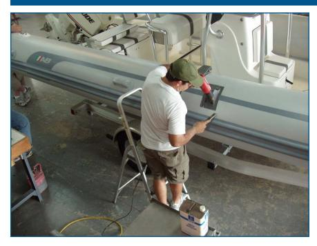
13. Curing the adhesive can be accelerated by carefully using a heat gun and a smooth rounded putty knife.
