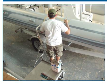
8. Apply 2 coats of the adhesive to the bonding surfaces on the boat, using a 2" (50.8mm) soft bristle paint brush, with the bristles trimmed to 3/4" - 1" (19 - (25.4mm) long.
