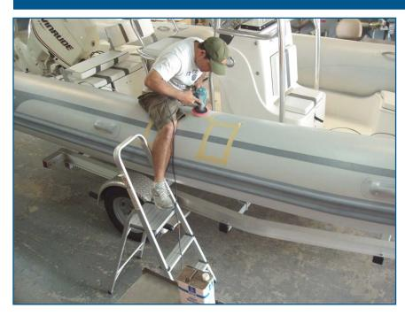
6. Rough the bonding surfaces on the boat with 120 grit sandpaper, using a rotary or flap sander.
