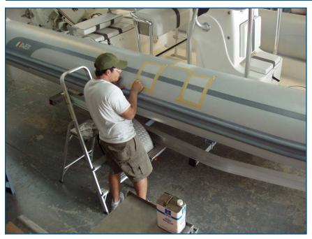
7. Thoroughly clean the bonding surfaces on the boat with solvent.
