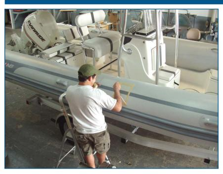
10. Wait until the adhesive is no longer "tacky". A quick test is to put your knuckle against the adhesive. If the adhesive doesn't transfer to your knuckle, remove the tape from the boat bonding surfaces.
