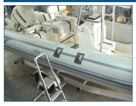
16. Completed installation of the snaps and hook, ready to receive the RIB Ladder.
