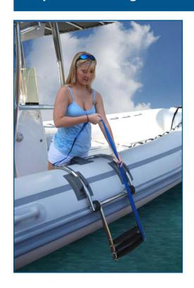
5. Lower the steps into the water, using the strap.
