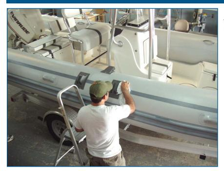
15. Clean off any excess adhesive to make a nice, clean, professional installation.
