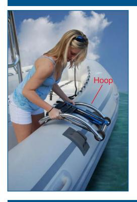
1. Position the hoop of the ladder underneath the hook. The radius (curve) of the hoop, should match the tube of the boat.
