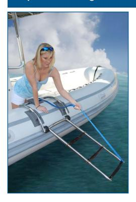
6. Pull the steps out of the water, using the strap.
