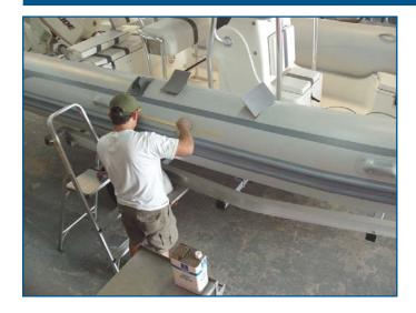
5. Tape off the mounting locations for the snaps and hook on the boat using masking tape.
