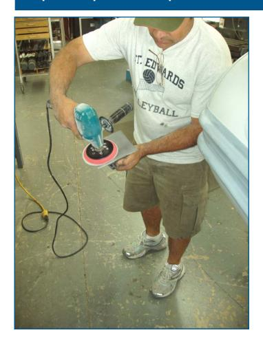
3. Rough the bonding surface on the snaps and hook with 120 grit sandpaper, using a rotary or flap sander.
