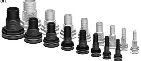
The Skin Fitting with Tail body and nut are moulded from glass fibre reinforced nylon composite. High strength, high-modulus glass fibres impregnated into the nylon provide dramatic strength, stiffness, toughness and dimensional stability. These properties allow a significant weight reduction over metallic fittings.
