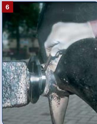
**6:** Assemble both halves of the unit round the shaft and align the locking grub screw with the drilled indent on the propeller shaft. Now firmly tighten both clamp bolts.
