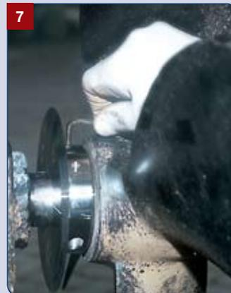
**7:** Firmly tighten the locking grub screw with one of the Allen keys and finally re-check the tightness of the two clamp bolts – that completes the installation work.
