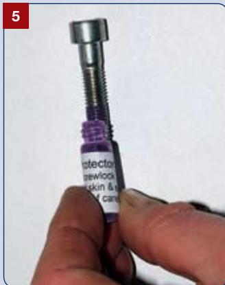
**5:** Carefully apply the thread-locking compound to the two clamp bolts. When both are screwed tight, this will help to keep them in place over time.
