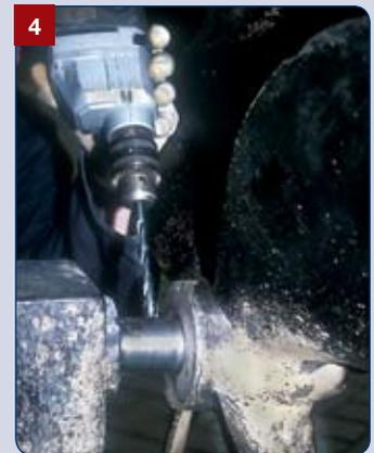
**4:** Remove the sharp blade, taking care not to cut yourself, and drill a shallow indent into the shaft where you marked the hole, in readiness for the locking grub screw.
