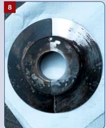
**8:** Following a tangle-free year since installing the ProProtector, I removed the unit for cleaning with wire wool and re-fitted it with fresh thread-locking compound.
