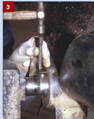
**3:** First, offer up the half of the blade underwater, the thread-locking compound won't cure, so an optional set of self-locking fastenings is available.
