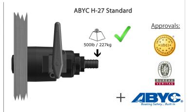
**ABYC H-27 requirements;** a 500 lb (226.8 kg) load is applied to the inboard end of the assembly (i.e. from the Tail fitting) for a minimum of 30 seconds without any damage occurring.
