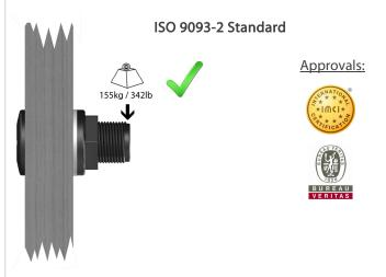
**ISO 9093-2 requirements;** a 155 kg (341.7 lb) load is applied to the threaded section for a minimum of 30 seconds, without any damage occurring.
